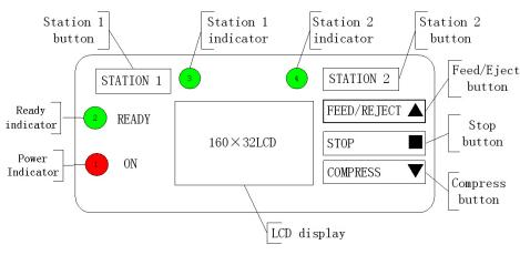
Figure 2.1-1 operator panel on printer
