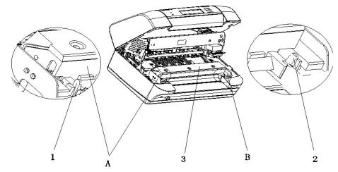
Figure 11.5-2 description of alignment unit
